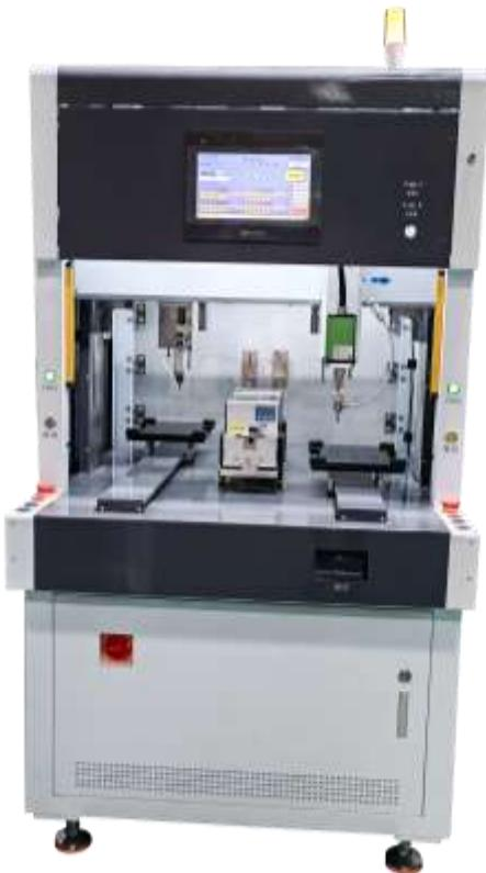
**Advantages & Highlights: Back-to-Back 6-Axis Dual Screwdriver Dual Station System with Alternating Operation Mode, boost productivity**
